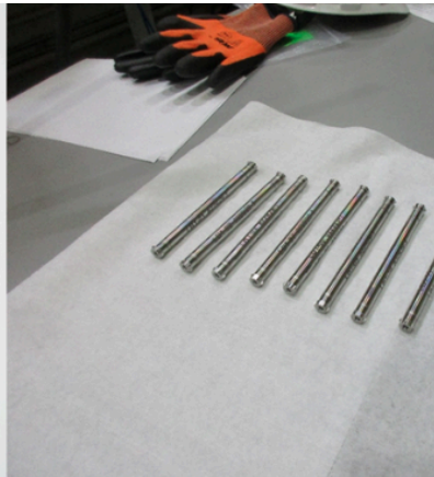
Capsules containing Lightbridge Fuel material samples before loading into an experimental assembly.
