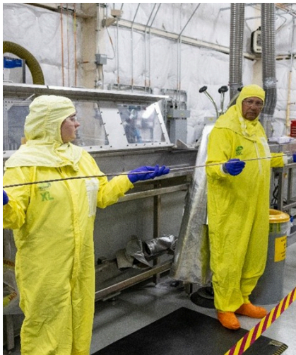
Enriched Uranium– Zirconium Rod Post- Extrusion
