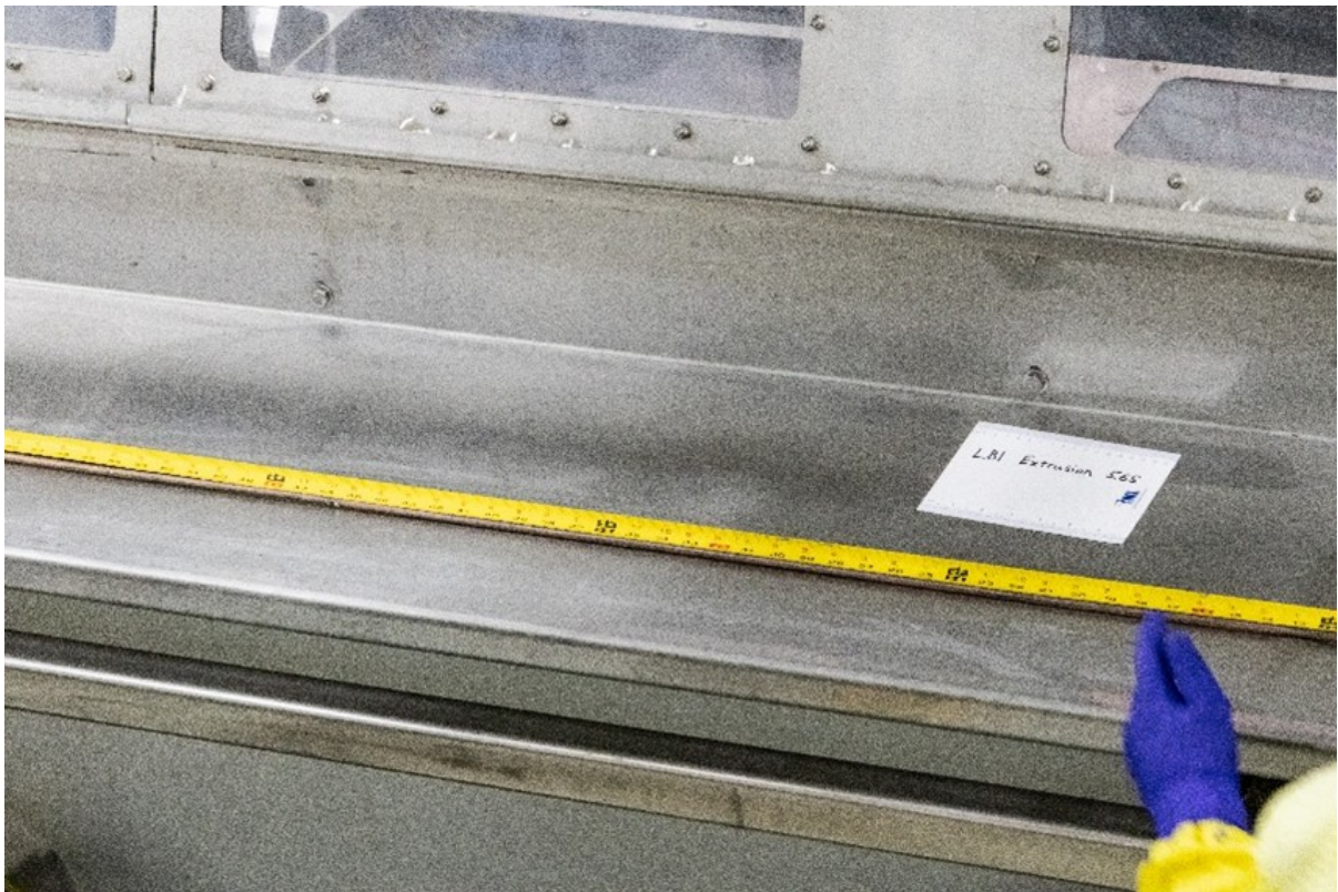
Image 3: Taking Measurements of the Enriched Uranium-Zirconium Rod Post-Extrusion
