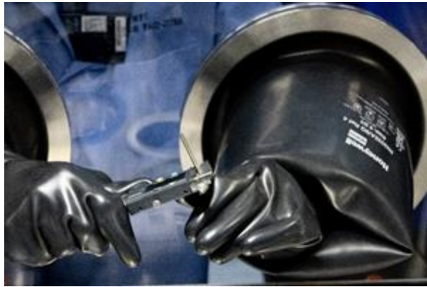
Taking dimensional measurements of a finished enriched uranium-zirconium coupon sample
