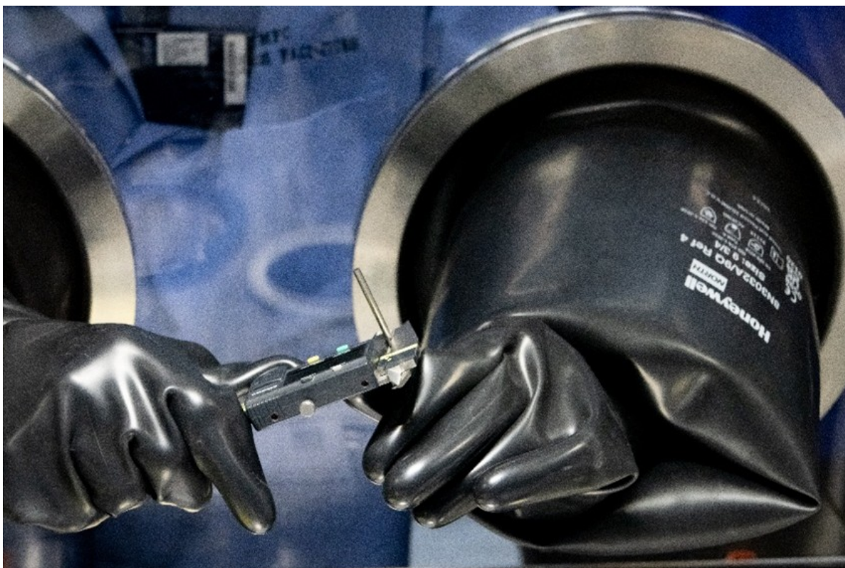
Image 7: Taking dimensional measurements of a finished enriched uranium-zirconium coupon sample
