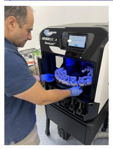
Advanced Dental Technologies, a fullservice lab based in Boston, recently purchased the new J3 DentaJet printer and has been using it to produce crown and bridge, removable, and implant models.
