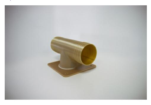
Final, flight-approved, 3D printed ducting for air conditioners. 3D printed in ULTEM™ 9085 resin on the Fortus 450mc (Photo: Business Wire)
