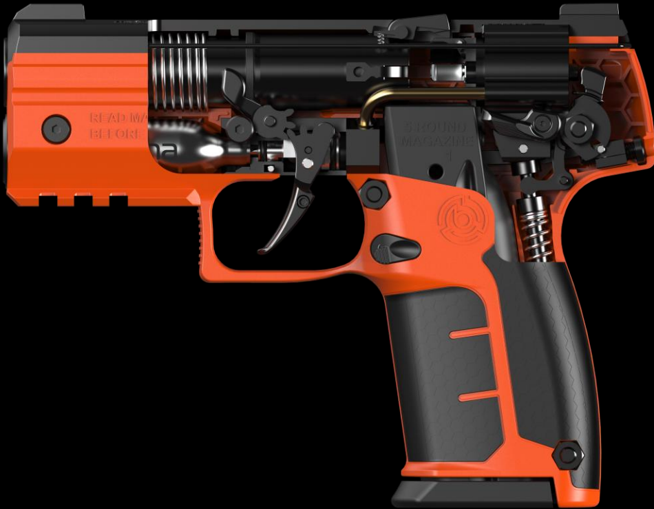
Byrna SD – Internals Cutaway
