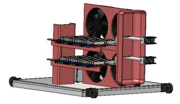
B-TRAN<sup>™</sup> based MVDC solidstate circuit breaker rated at 12 kV, 500 A (6 MW)
