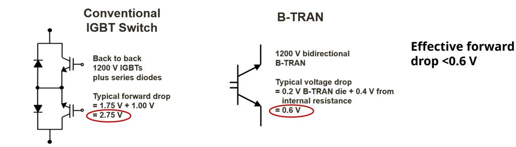
Conduction Losses in Bidirectional Applications >4x better than IGBT + Blocking Diode
