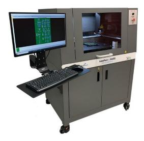
AP-MARS fully automates circuit card troubleshooting and schematic generation, significantly reducing human error and time to repair.
