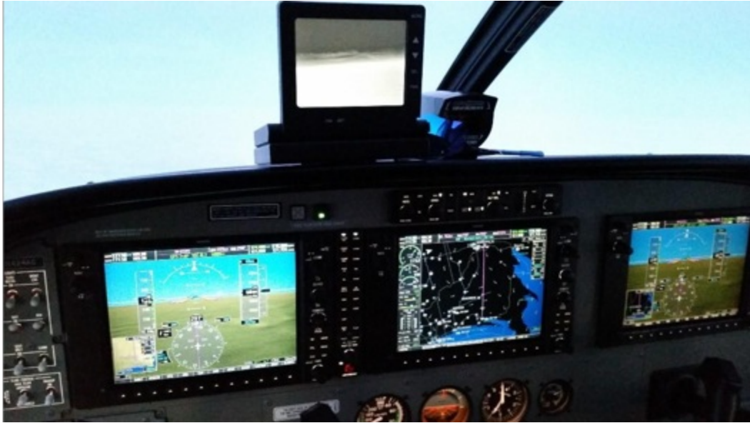
Max-Viz 600 EVS displays on a flipper screen above the glare shield.
