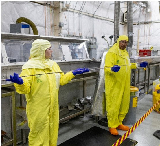
Enriched Uranium-Zirconium Rod Post-Extrusion
