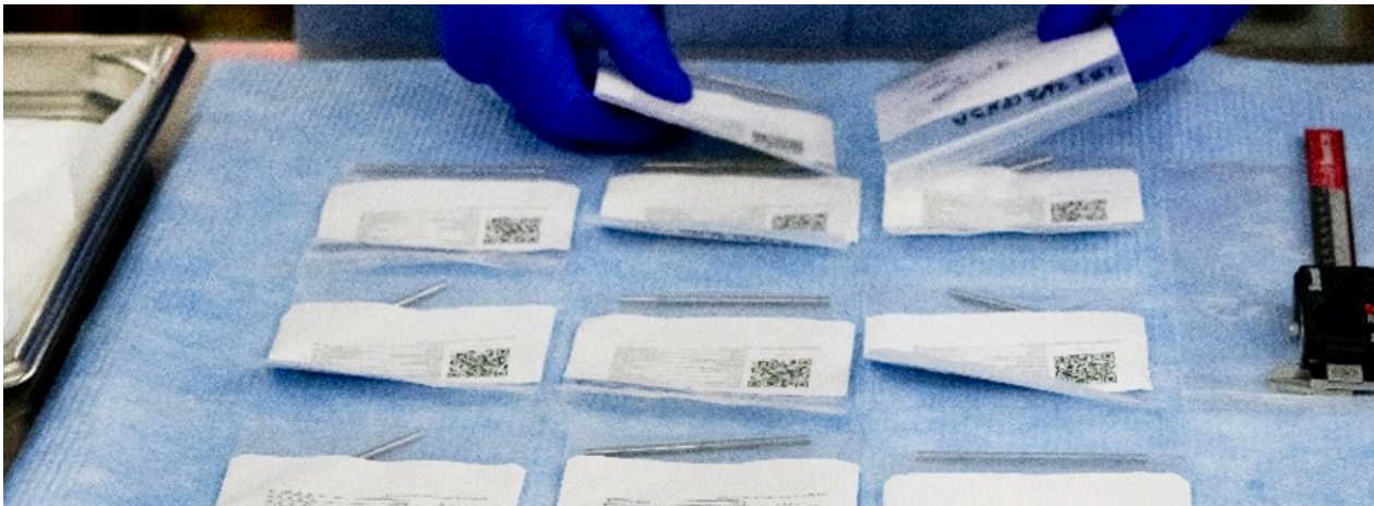
Finished enriched uranium-zirconium coupon samples after characterization and visual inspection results confirmed their suitability for irradiation testing in the Advanced Test Reactor
