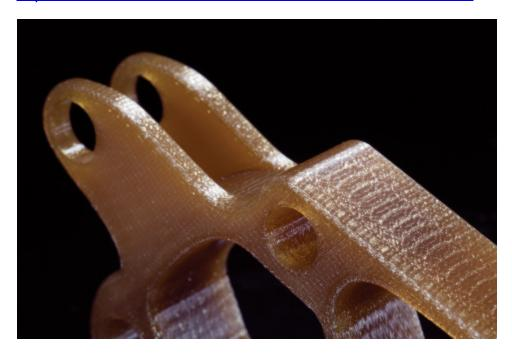
Stratasys' Antero 800NA thermoplastic produces 3D-printed parts with the toughness and chemical resistance needed for many aerospace applications. (Photo: Business Wire)
