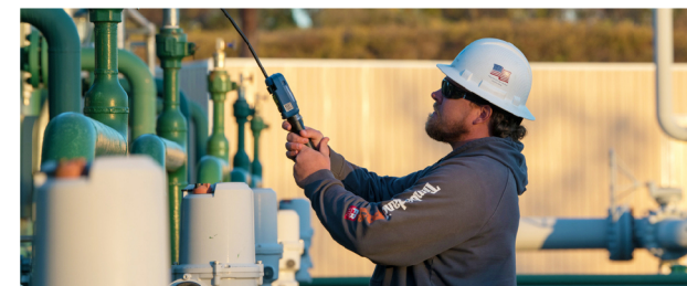
Handheld emissions detection devices in the hands of every field operations employee support our zero-tolerance policy against fugitive emissions.
