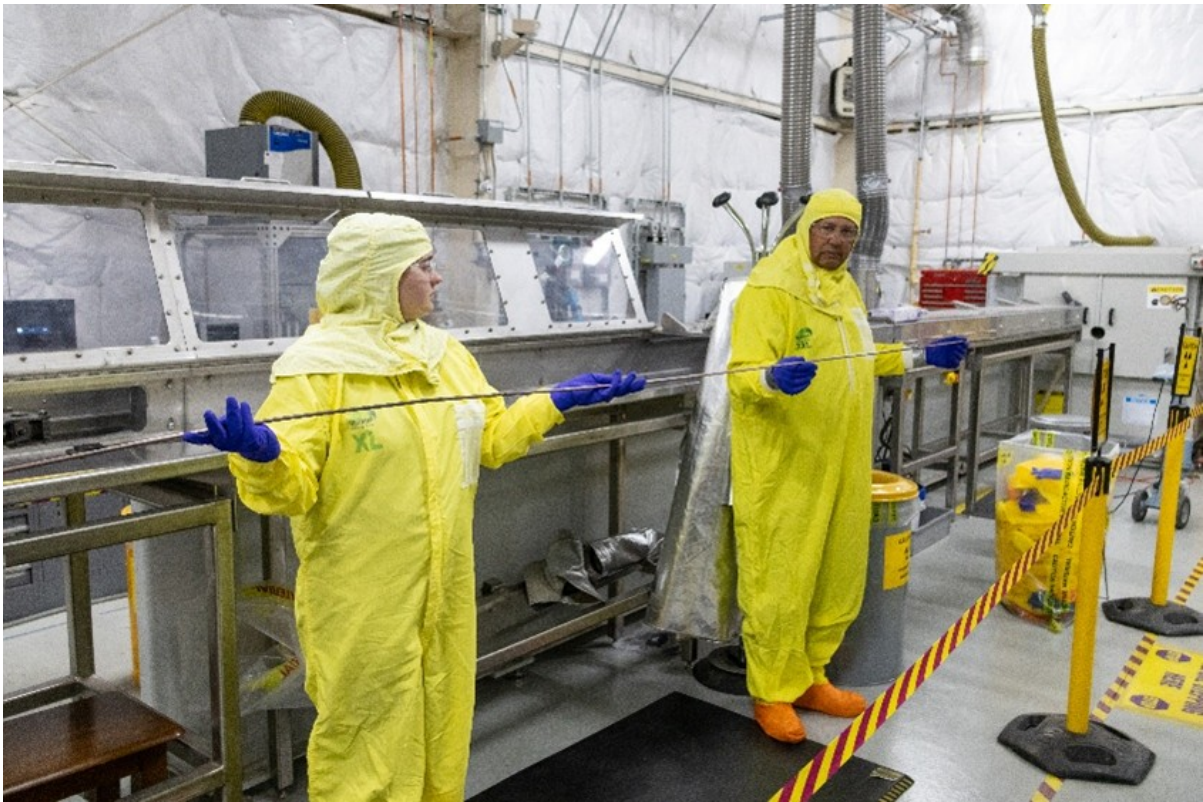
Image 1: Enriched Uranium-Zirconium Rod Post-Extrusion
