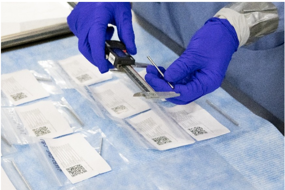
Image 10: Taking dimensional measurements of a finished enriched uranium-zirconium coupon sample
