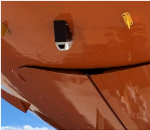
Max-Viz 1400 installed on DC-10
