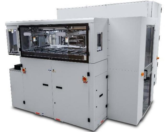
The new ATS 5034 SLT Platform delivers a high throughput and low cost of test for testing semiconductor devices at the system level.
