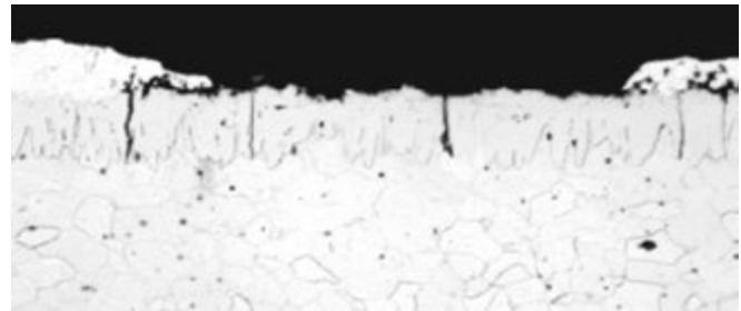
Coating Pit on 30-year old pipe demonstrating arrested pit penetration.
