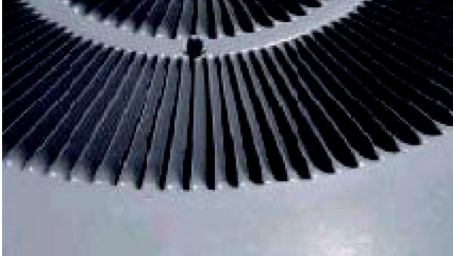
1.0 mil Prepainted Louvers after 16 months Daytona Beach exposure (fan running).
