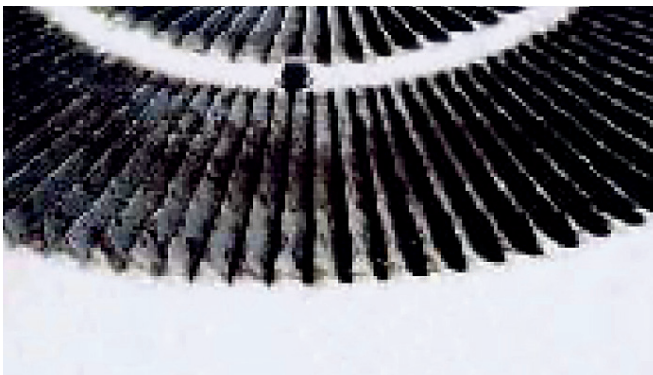
1.0 mil Prepainted Louvers after 16 months Daytona Beach exposure (fan running).
