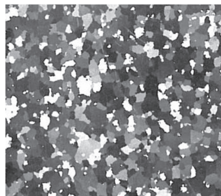
Sample chemically etched to reveal grain structure.
