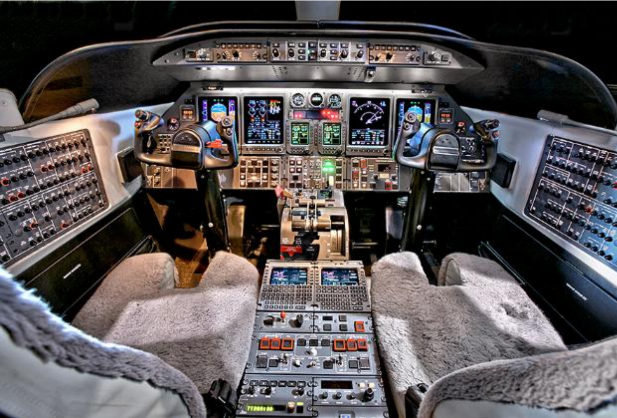
Traditional Cockpit with Mechanical Circuit Breakers Learjet 45
