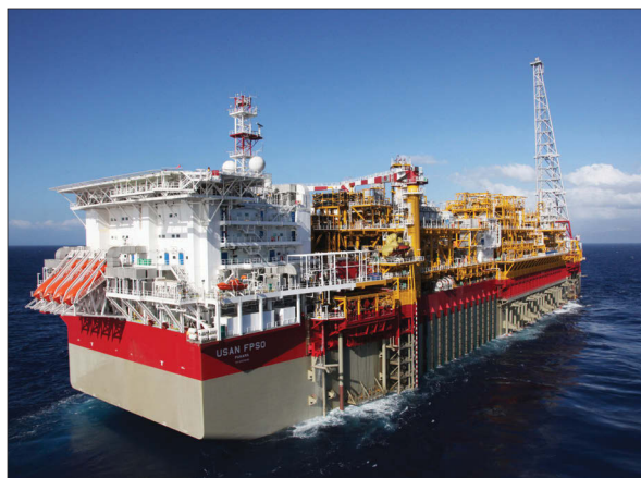
Our Usan development offshore Nigeria utilizes subsea wells tied back to an FPSO vessel.
