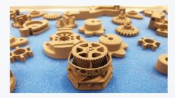
"With the Shop System, PORAL is able to deliver breakthrough productivity, precision, and surface quality by combining the flexibility of 3D printing (design freedom, elimination of tooling, and sustainability) with the advantages of powder metallurgy (quality, repeatability, and energy savings). Our products are engineered to withstand the harshest environments, and additive manufacturing via binder jetting is a critical step in advancing the state of the art." -Denis Pugnet, CEO
