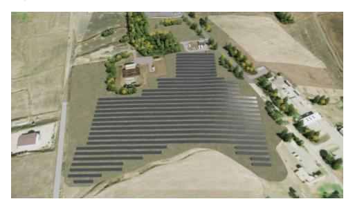
Rendering representative of the USCG Training Center Petaluma partnership with cleantech integrator, Ameresco, to install a microgrid, integrating existing distributed backup generators with a new 5 megawatt (MW) solar array and an 11.6MWh BESS to power the entire site in the event of a loss of utility (LoU). (Photo: Business Wire)
