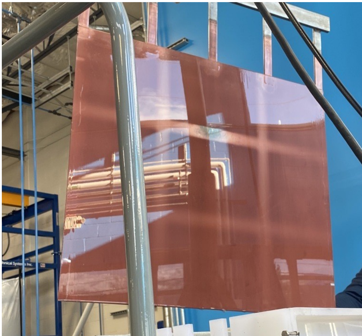
A modular, production-scale copper plating Aqualyzer, with the first plated battery metal, at Aqua Metals’ pilot facility
