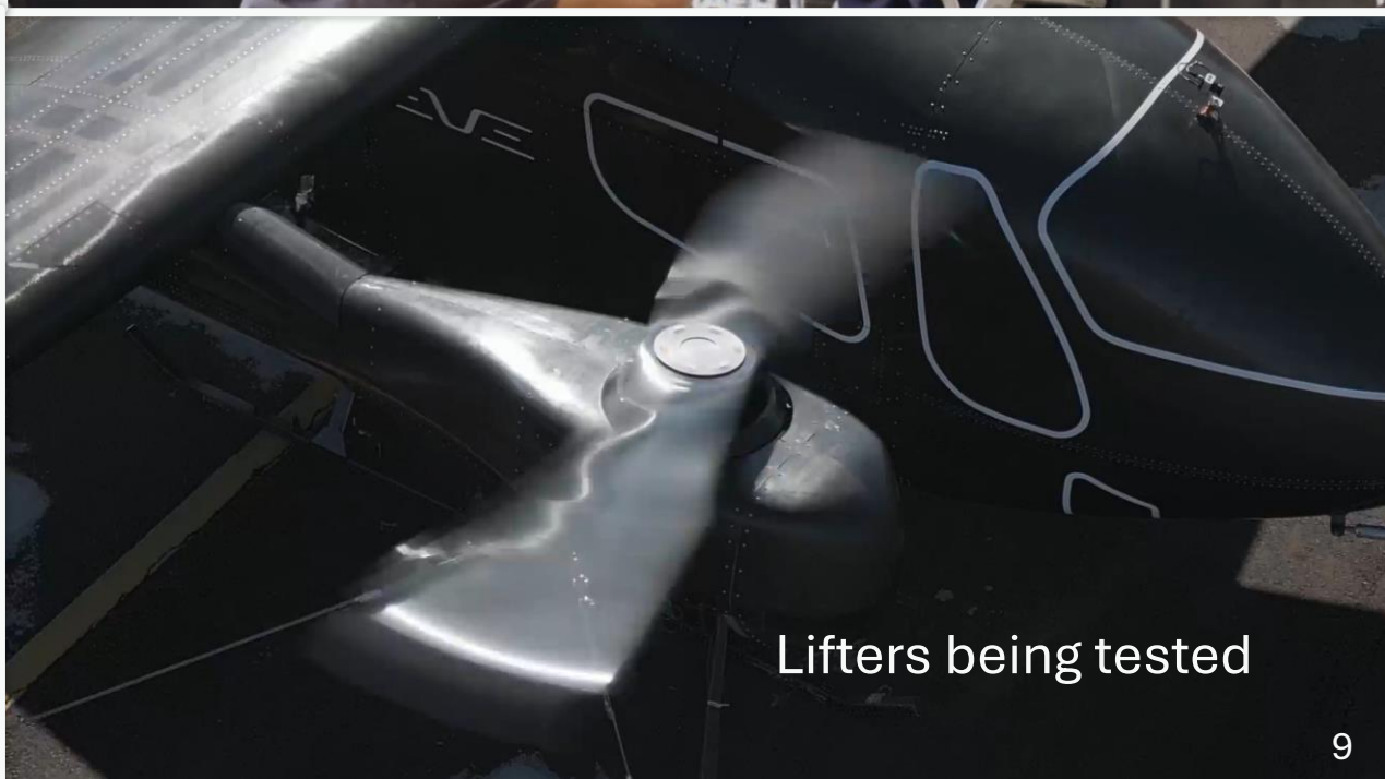
Mobile rig run tests to check the blades in flight speed
