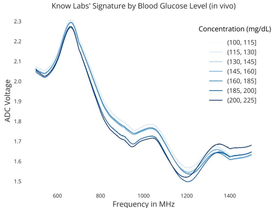
The signal received is modified due to the **dielectric properties of blood glucose**
