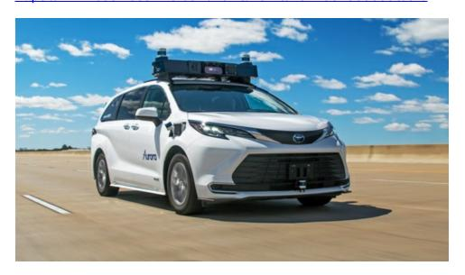
Aurora unveiled its test fleet of its autonomous custom-designed Toyota Sienna vehicles featuring Toyota's Vehicle Control Interface (VCI) and "Sienna Autono-MaaS" (S-AM) platform. (Photo: Aurora)
