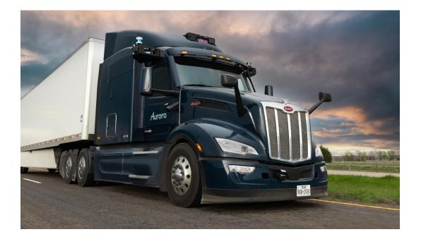
Despite a rigorous calibration process and the high level of ruggedization of our sensor pods, miscalibration caused by mechanical fatigue, thermal drift, or even impacts with flying debris is always possible during a truck's journey. To address this, our team has developed an online calibration system which enables the Aurora Driver to detect and measure miscalibrations and recalibrate while on the road. These real-time calibration system is consistently high-performing when on the road.
