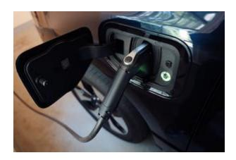
F-150 Lightning's bidirectional design allows the vehicle battery to both charge and then discharge energy back to the grid when it's needed most.
