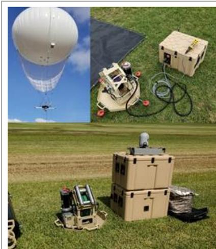
Drone Aviation's new ultra-tactical WASP Lite aerostat system is easily transportable and deployable from a series of ruggedized cases.
