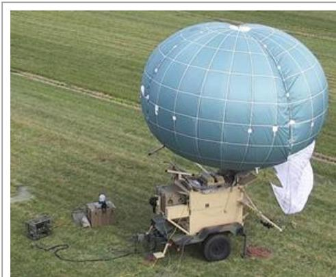
Drone Aviation's Winch Aerostat Small Platform ("WASP") is a highly tactical and mobile aerostat system which can be operated by as few as two soldiers and can provide day/night video, secure multi-frequency and multi-wave form wireless communication range extension capability at the edge of the battlefield from either a stationary position or while being towed.
