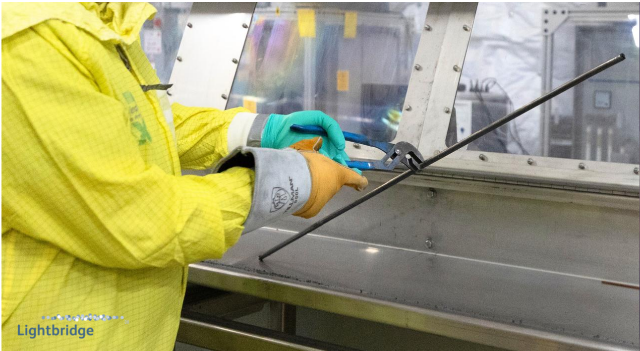
URANIUM-ZIRCONIUM ROD POST-EXTRUSION:
