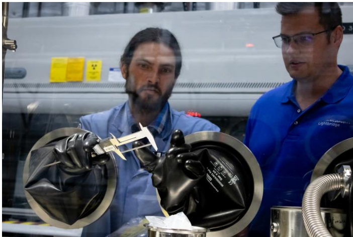
Lightbridge and INL Team Performing a Visual Inspection of a Finished Enriched Uranium-Zirconium Coupon Sample inside a Glovebox
