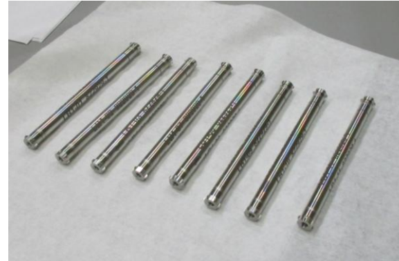
Capsules containing Lightbridge Fuel material samples before loading into an experimental assembly.
