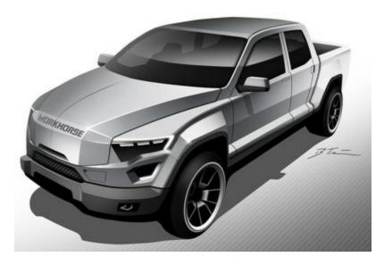
Expected to be in production 2018, the new Workhorse W-15 light duty platform design is an extension of the E-Gen electric technology used in Workhorse medium-duty delivery trucks. With an expected 80 mile battery range using Panasonic 18650 Li-ion batteries, the Workhorse W-15 light duty design expects to provide economical, clean and powerful performance.
