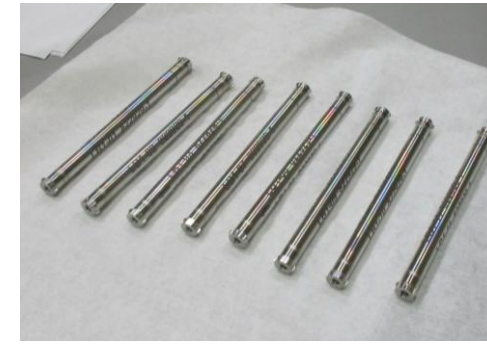
Capsules containing Lightbridge Fuel material samples before loading into an experimental assembly.
