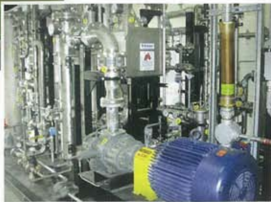
Biogas is conditioned in the BioCNG unit (below), then routed to a CNG fueling station (left) where it is further dried and compressed for vehicle fueling.
