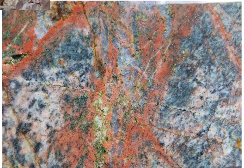
Figure 6. Gray, strongly-foliated granodiorite with limonite on fracture surface.
