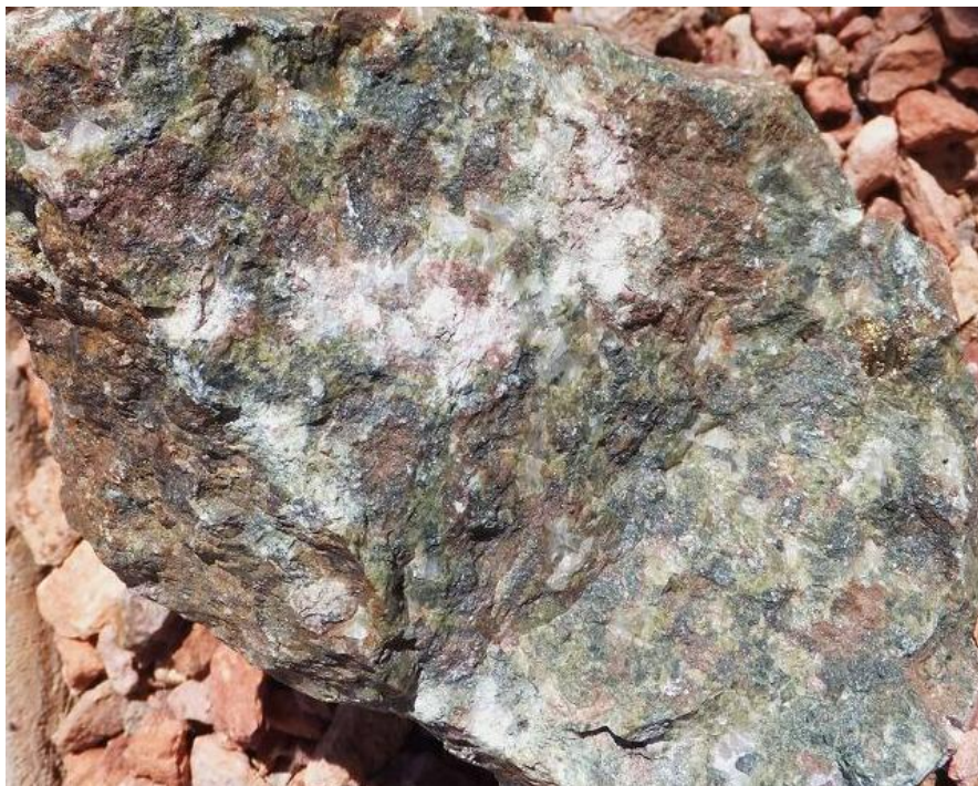
Figure 9. Pervasive propylitic altered Sherman Granite (?) at the Rambler anomaly. The original rock was replaced by epidote, chlorite, calcite, hematite and primary sulfides including chalcopyrite, pyrite, sphalerite and minor specularite.
