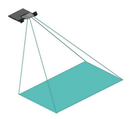
MicroVision's PSE-0403sti Interactive Display Engine has a short throw ratio producing images with nearly 2 times the diagonal width of the height of the device. (Photo: Business Wire)
