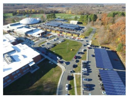
Wayland's solar arrays are comprised of a total of 4.214 photovoltaic panels totaling 1,289 kW, and designed to generate over 1.5 million kWh of renewable electricity each year. Collectively, the three solar canopies at the High School, Middle School and Town Building, in addition to a roof top system at the Department of Public Works building are expected to generate enough
