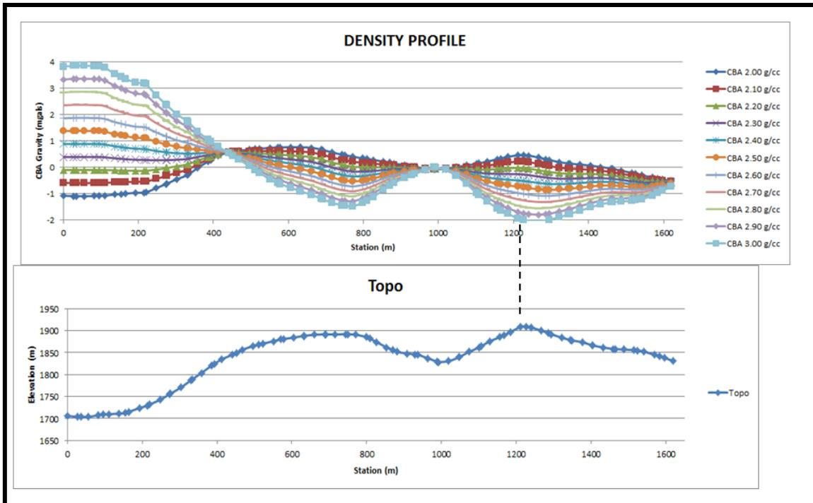
**FIGURE 4: Density Profile CBA and Topographic Profile (Sections Look Northwest)**
