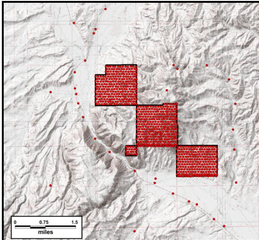
*FIGURE 2: Maggie Creek Gravity Station Posting*
