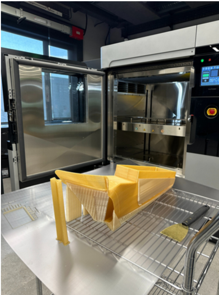
A composite layup tool, printed on a Stratasys F900. (Photo: Business Wire)
