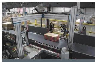
Multiple integrated distribution and fulfillment systems (including laser-based identification and dimensioning technologies) communicate in a warehouse to identify and route items and parcels through the facility and out to a customer.
