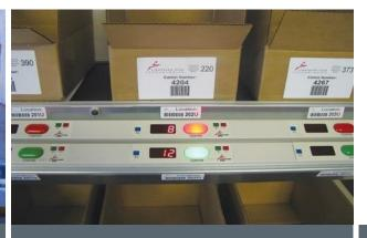
Industrial's **Pick-to-Light Systems** utilizing light indicators for sorting and control of merchandise.
