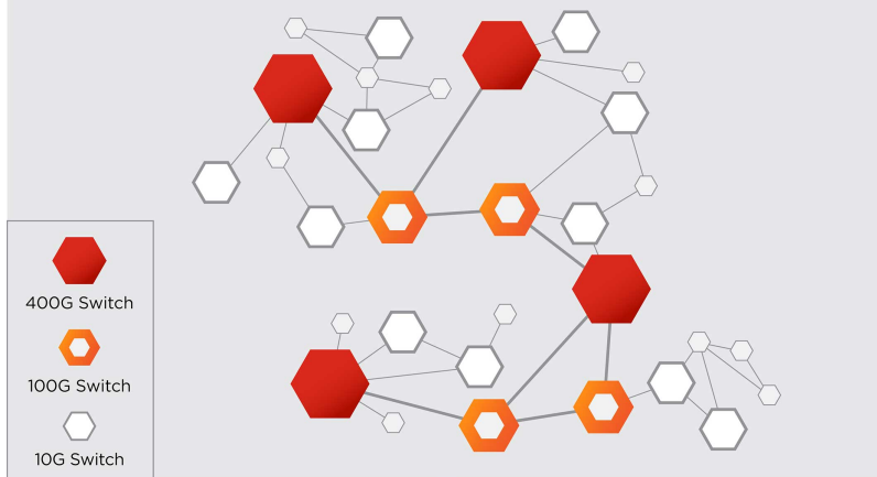
Traditional Ethernet deployment, with many different scale and port density switches
