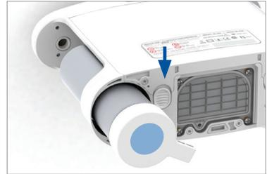
8. Remove the column (metal tube) completely from the Inogen One® G3.
