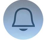
Breath Detection Alert Mode. The Inogen One® G3 will alert with audible and visual signals for “no breath detected” when this mode is enabled and no breath has been detected for 60 seconds. At 60 seconds, the device will enter into auto pulse mode and once another breath is detected, the device will exit auto pulse mode and deliver normally on inspiration. The display’s mode indication area will show a bell icon, flashing red or yellow light and display message when the alert is enabled.
