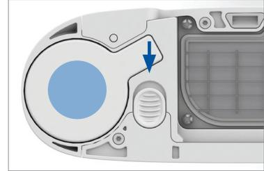
7. While holding the button open, slide the column (metal tube) out by gripping the exposed aluminum surface with other hand.
