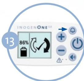
Press the alert/bell button once and screen will display "sieve reset success." Press the power button to turn on the Inogen One® G5, and use normally.
