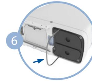
While holding the button open, slide the column assembly out of the device by pulling on the column pull handle.
