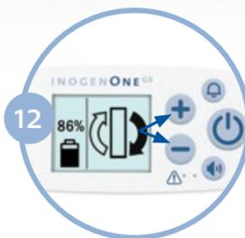
Press and hold the plus (+) and (-) minus buttons for 5 seconds. The screen will display "sieve reset" message. Release buttons once message is displayed on screen.
