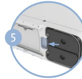
Unlock the column assembly by pushing the latch button away from the columns.
