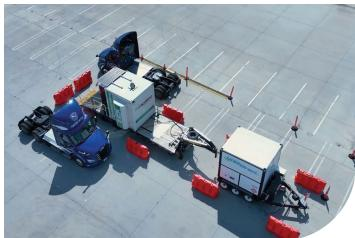
system combined a Capstone C200S microturbine with an onboard DC fast charger, providing up to 180 kW of continuous power. Designed as a fully off-grid solution, the mobile platform could charge two heavy-duty Class 8 trucks simultaneously without relying on utility service.
