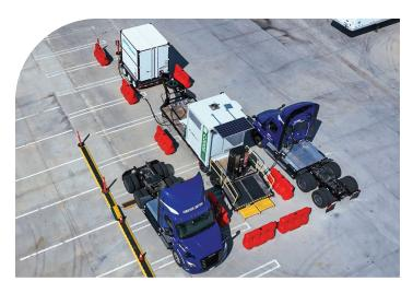
Capstone deployed its first trailer-mounted mobile EV charging unit, combining a C200S microturbine with an on-board DC fast charger to deliver 180 kW of continuous, off-grid power. The platform charged two Class 8 electric trucks simultaneously without relying on utility service, giving the customer a clean, flexible solution to accelerate fleet electrification.
