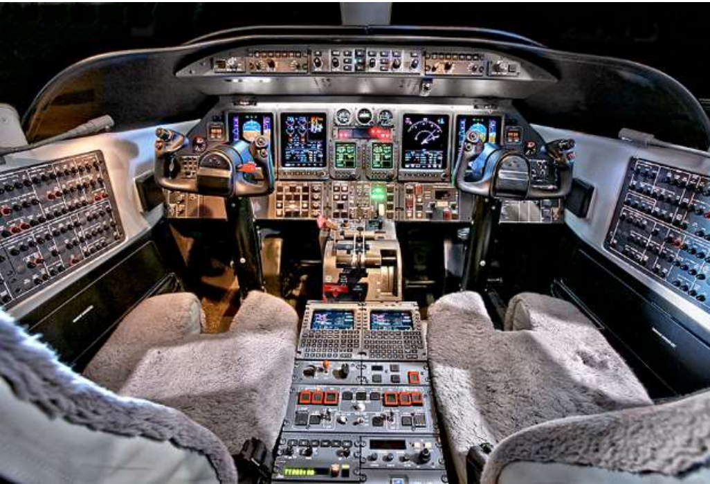
Traditional Cockpit with Mechanical Circuit Breakers Learjet 45
