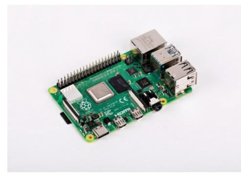
The MxL7704 complete power delivery system already powers the popular Raspberry Pi 3 Model B+. The versatility of this universal PMIC allowed it to be easily re-programmed to accommodate the new current limit. sequencing and power requirements of the upgraded SoC and surrounding ICs on-board the new Raspberry Pi 4.
