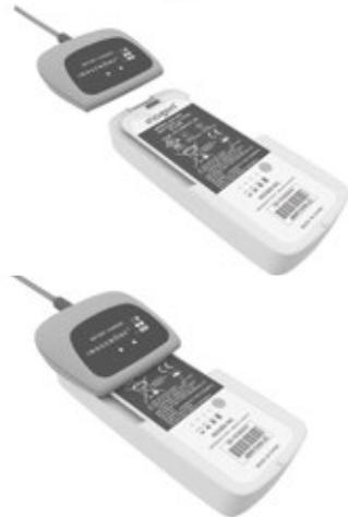
**NOTE:** These contacts are not powered unless a battery is in place and charging. To completely remove power from the external battery charger, remove the plug.
