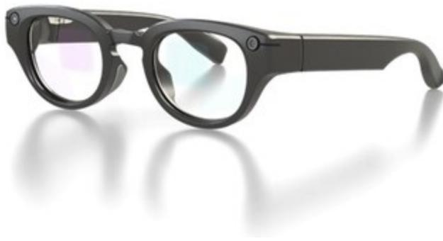
The reference design integrates Avegant's AG-30L3, a breakthrough 0.7 cc full-color LCoS light engine, with Vuzix' advanced waveguide optics, delivering bright, crisp, full-color imagery in an ultra-compact form factor. The platform enables OEMs to accelerate development of both consumer and enterprise AR smart glasses by offering a ready-to-manufacture architecture that significantly reduces size, weight, and total system cost.
