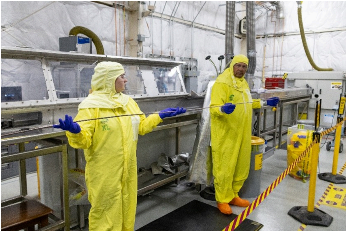
Image 1: Enriched Uranium-Zirconium Rod Post-Extrusion
