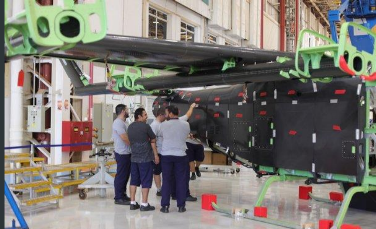
COMPOSITE FUSELAGE "SKIN", WING, PYLONS AND NACELLES, STARBOARD SIDE
