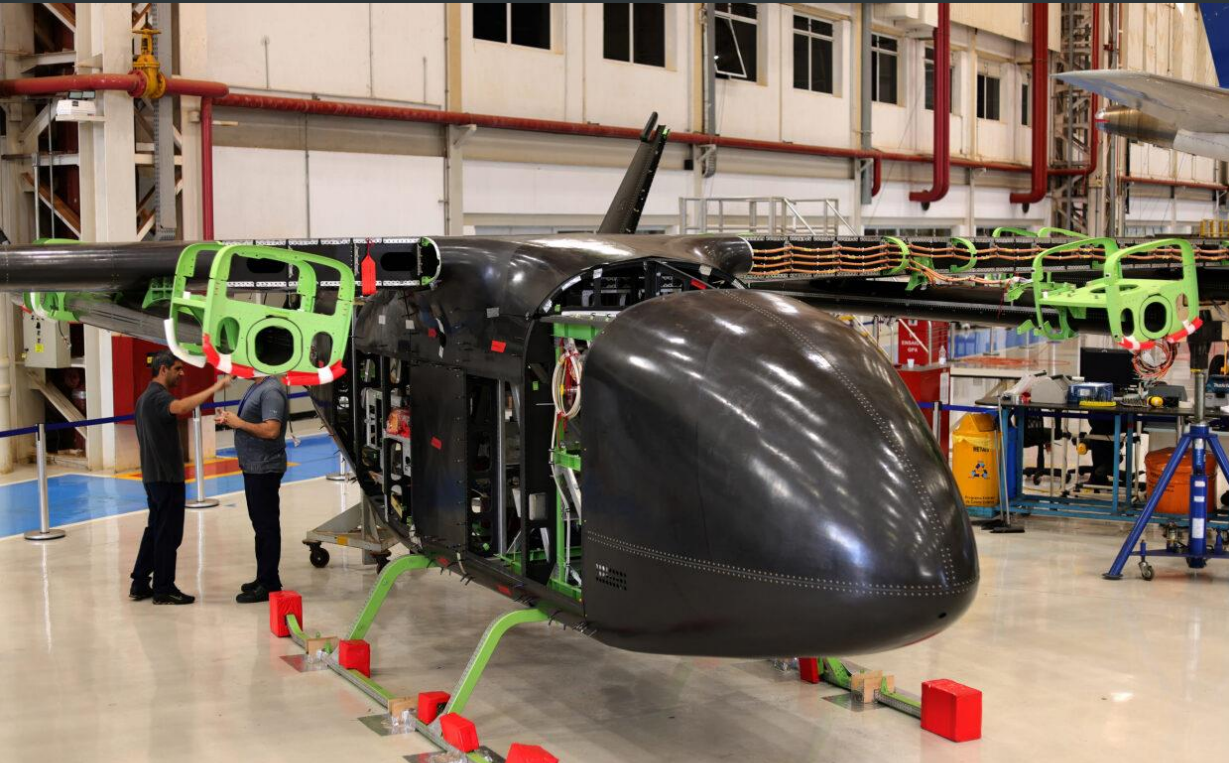
COMPOSITE FUSELAGE "SKIN", WING, PYLONS AND NACELLES, STARBOARD SIDE
